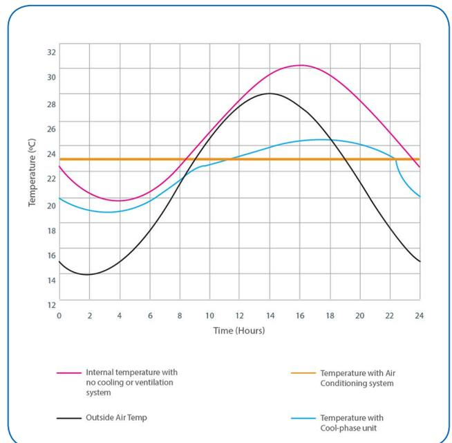
The **orange line** shows the effect a high energy system such as air conditioning or similar would have if it was set to a 23°C cooling set point. The AC system would try to hold the room to 23°C but the temperature would still fluctuate by a degree or two in reality.
