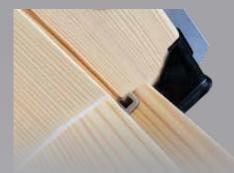
Special water drainage channels are introduced in the lower corners of the frame to discharge water from condensation and potential leakage caused by, e.g. damaged external aluminium profiles. Wooden profiles are less exposed to the moisture, which adds to their durability.
