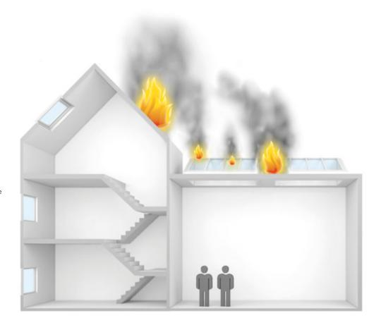
The tests assess the fire spread across the external surface of the roof\*, the fire spread within the roof\*, the fire penetration and the production of falling droplets or debris falling from the underside of the roof\*.
