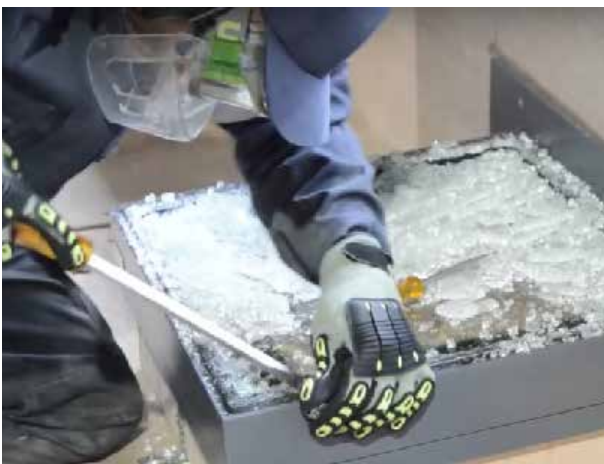
'Testing fixed Flushglaze rooflights in line with part Q building regulations'
