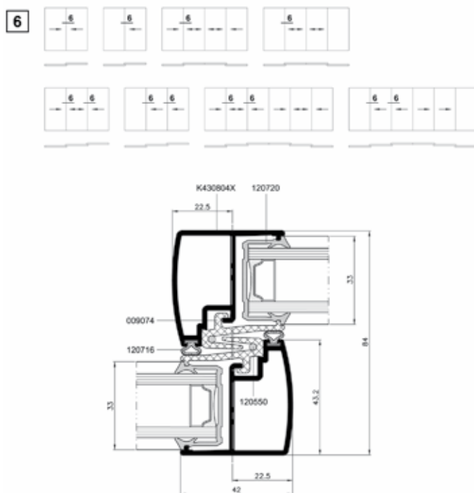
Cross-section of door and window jambs
