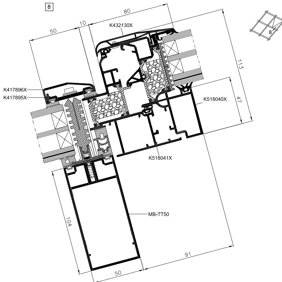
Transom and roof window - cross - section
