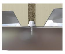
Opticore is EJOT's unique and patented integral nylon head, designed to encapsulate fasteners from our high performance self-drilling range. Opticore is engineered to provide a dual drive fastening system that enables rapid self-coring of membrane faced insulation panels, and a secure fix into hot and cold rolled steel, and timber.
