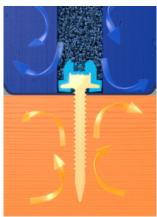
A combination of hot box tests and thermal activity recording at EJOT's testing centre Applitec, has repeatedly shown that the composition of the Opticore head provides significantly better thermal retention values over all-metal fastenings.
