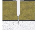
EcoTek with FPS-E aerated concrete screw
