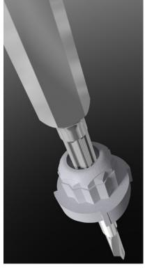
The intergral Opticore head design is manufactured in high strength moulded nylon. The 'cutting fins' are unique to the Opticore patent, and create the smooth coring of the panel's insulation. On secure 'pull-up' of the fastener into the substrate, the fins simply snap away without any compromise to the integral lining.
