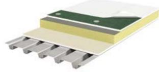
Cover boards can also enhance durability in roof systems using mechanical fasteners rather than adhesives. In these systems, wind forces may try to rock the fasteners sideways, and the fasteners can lose compression or even back out of the decking. A suitable cover board under the membrane can keep the fasteners from rocking and protect the roof.
