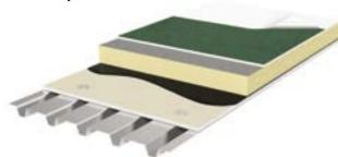
Where the waterproofing membrane is held down by a continuous coating of adhesive, wind performance relies on the strength of the substrate. If the waterproofing membrane is bonded directly to a low density insulation layer, uplift forces can pull the insulation apart.
