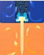
Hot box tests and thermal activity recording has repeatedly shown that the composition of the Opticore head provides better thermal retention values over metal
