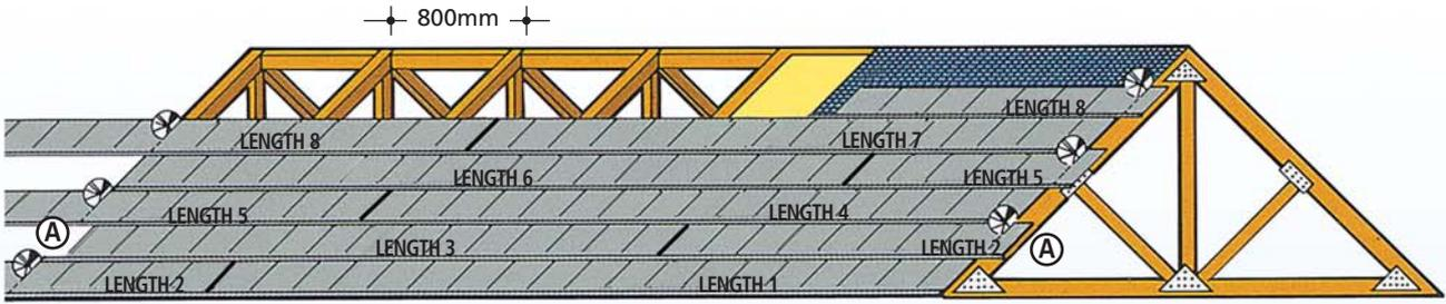
Meta-Slate is available in standard lengths. Using a combination of these, together with the joining plate it is possible to clad any length and shape of roof. The joining of two lengths does not have to coincide with a truss/rafter as the joined lengths form an extremely rigid joint.
