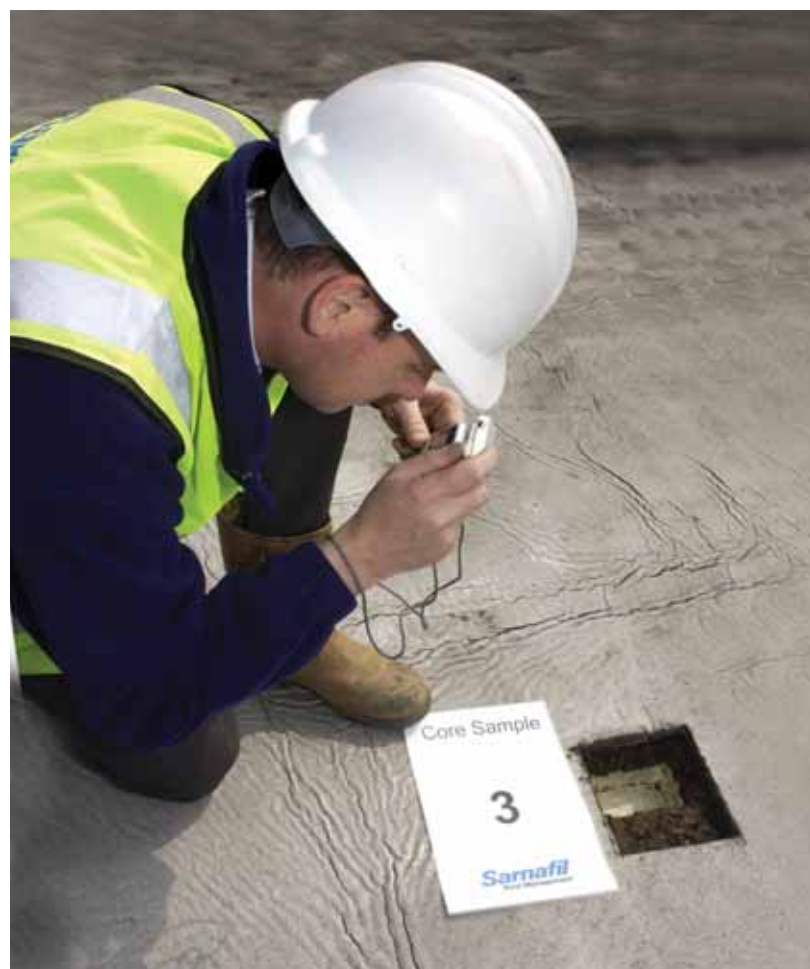
Core sample recording Photographic records being made for a roof survey report.
